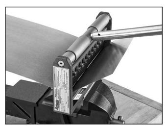
Figure 7. Example of a 90° bend.
